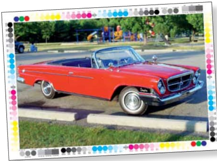
FIGURE 2 SINGLE AND SEVERAL-UP PROOFS The most common way to proof a color image is to use one absolute zero-tolerance color version that's been approved and promised to be matched visually. Digital proofing makes it possible to create controlled visual representations of press variations before the job gets to production.
