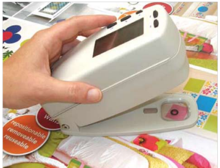
FIGURE 6 SPECTROPHOTOMETER READING You can use a spectrophotometer to read a match color using the visually determined color-tolerance numbers to establish a high and low reading for L*, a*, and b*.
