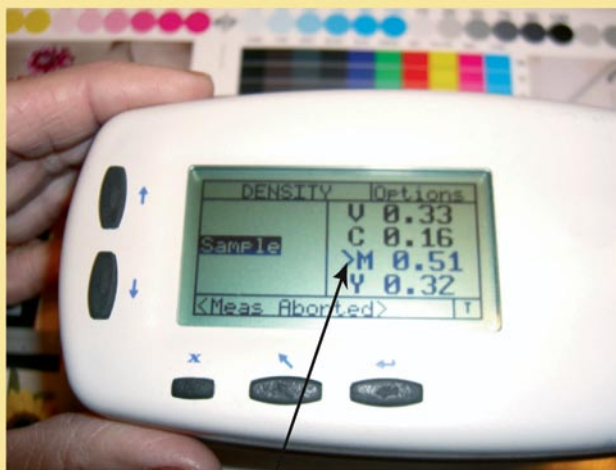
Dominant density is magenta, but notice that the other colors are reported too. This is very useful information.
