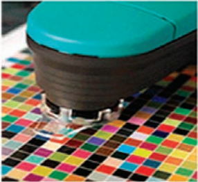
Calibration and colour measurement instruments have evolved for digital proofing systems, enabling greater accuracy.
